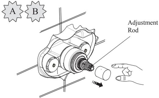
Remove the protective plastic cover without rotating the adjustment rod
