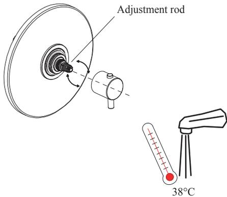
Ensure that the red dot on the temperature stop ring must align with the temperature position symbol (38) on the temperature control knob.
