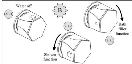
In 2.2.1 position the mixer does not provide any water
