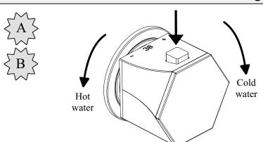
The button of the handle represents the temperature limit set up at 38° by the factory. To overcome this limit you have to push the button and turn counterclockwise, while to reduce the mixing water temperature you have to turn it clockwise.
