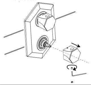
Turning the adjustment rod with the help of a clamp (pay attention not to damage the rod) up to the 38° C temperature. (thermometer)
