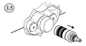
Unscrew the cartridge with a 24 mm key and pull it out from the mixer body.
