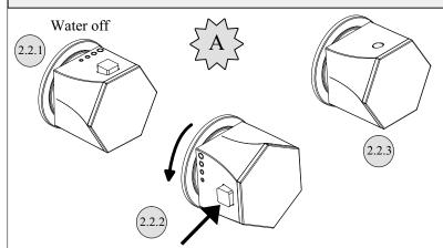
In 2.2.1 position the mixer does not provide any water.
