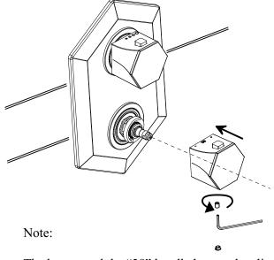
The button and the "38" handle have to be aligned at 12 o'clock before assembling.
