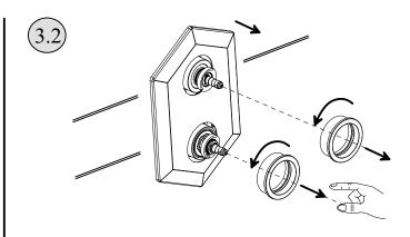
Unscrew the fixing shrouds counterclockwise and then remove the plate.
