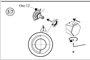
Put the white plastic cam "as shown in picture on the left" so that the landmark is at 12 o'clock position with respect to the body of the mixer.
