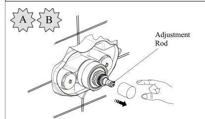
Remove the plastic protection without rotating the adjustment rod
