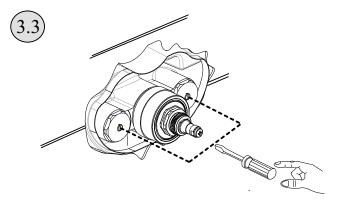
Close the water supply screwing clockwise the screws on the plugs of non return valves using a screwdriver.
