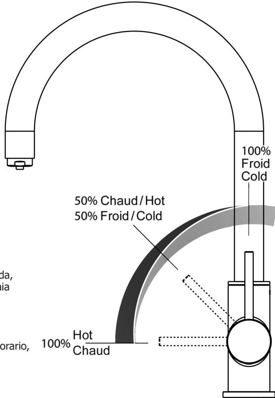
With **EnergySave** System, when opening with lever in vertical position the mixer delivers cold water only, thus preventing the water heating system from starting. This grants a significant benefit in energy and cost saving.
